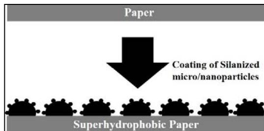
Fig. 1 Process flow of fabrication of superhydrophobic surface
