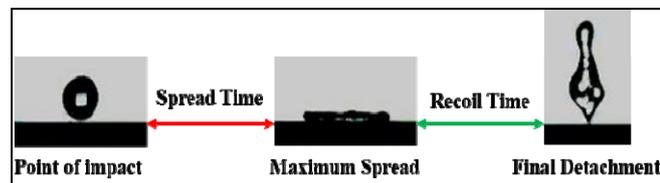
Fig. 6 Spread time and recoil time during drop impact on superhydrophobic surface
