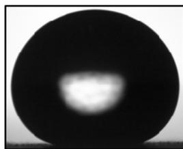
Fig. 4 Water droplet on superhydrophobic paper surface
